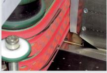
Siegling Linpack folder and carrier belts (with natural rubber Linatex coated power transmission belts) are used in the paper industry and letter sorting and elsewhere as pick-off belts.
